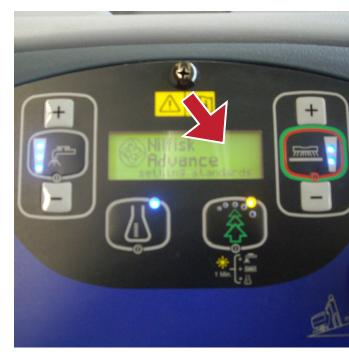
2 Check if there isn't any brush motor 3 overload i.e. 3 battery Ledsflash simultaneously or error code on dis-
