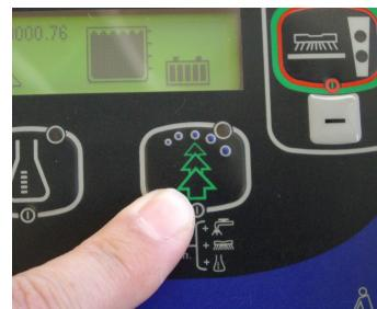
9. Press the EcoFlex™ switch whenever you temporarily need a greater cleaning power.
