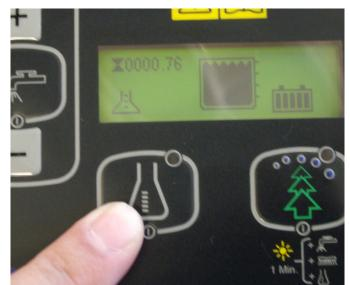
8. Press the detergent flow control switch. The number of display shows the detergent concentration level in the solution (see the table on the label). See the User Manual for setting change.
