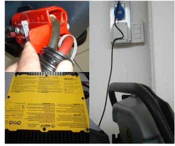
18. Charge the batteries: Connect the battery charger cable from the electrical main.
