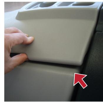
Close the recovery tank cover properly and/or verify the gasket wear.
