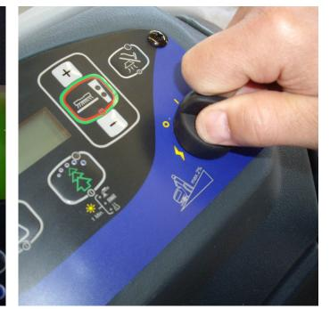
**3** Turn the ignition key to "0", then try to start the machine without pressing the paddle.
