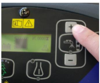
7. Press the solution flow control switches as necessary, depending on the type of cleaning to be performed.
