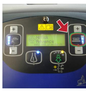
Check if the Leds are on. Wait until the lights are steady.
